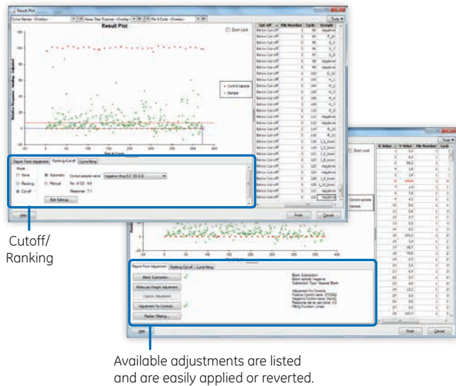
Fig 10. Using Result Plot , up to 5000 samples from several runs can be co-evaluated enabling easy selection of the samples of interest.
