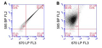
**Figure 2.** THP-1 cells labeled with dsRed-conjugated antibody show strongest signal in FL2 (585/40 BP) of the C6, but also show significant signal in FL3 (670 LP). Uncompensated data (A), Compensated data (B, FL3 – FL2 = 83%)
