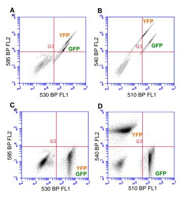
**Figure 1. GFP** and **YFP** signals are both detected in FL1 using the standard C6 filter configuration (A, C), but can be separated using the 510/15 filter (CP-170) in FL1 and the 540/20 filter (CP-178) in FL2 (B, D). Plots A and B are uncompensated data; plots C and D are compensated.
