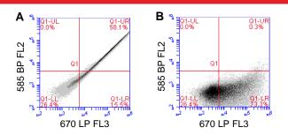
**Figure 4.** 293T cells transfected with mCherry show strongest signal on FL3 (670 LP) but also have a significant signal in FL2 (585/40 BP). Uncompensated data (A), Compensated data (B, FL2 – FL3 = 25%)
